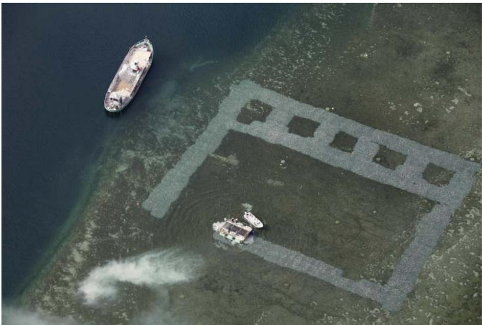
FIGURE 3 Aerial view of the lattice-structured gravel covering in Sipplingen Bay.
