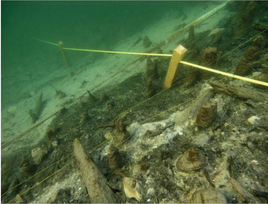
FIGURE 5 Reference posts for monitoring erosion on Greifensee (Canton of Zürich). The tape measure and lines attached to the stake for monitoring purposes are easily recognizable. *Photograph Amt für Städtebau Zürich — Unterwasserarchäologie*
